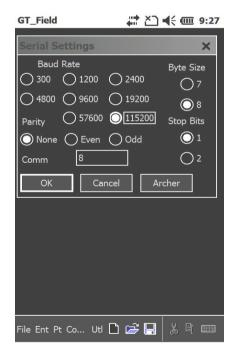
The Nikon C-100 is not configurable on the instrument, and operates at 4800 Baud, No Parity, 8 Data Bits and 1 Stop Bit, so you will need to set your HPC to match these settings.
